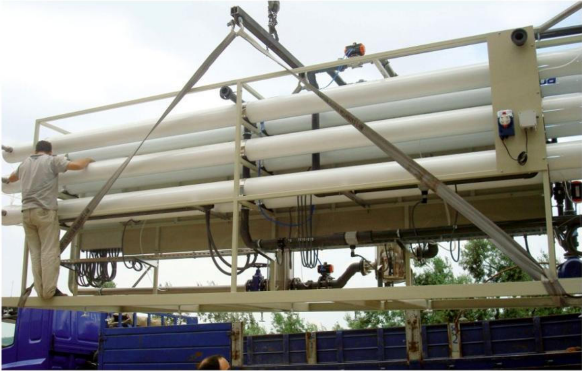
REVERSE OSMOSIS UNITE MARTUR AUTOMOTIVE - KÜTAHYA / TURKEY
